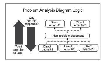
If there are two or more causes combining to produce an effect, they are placed at the same level in the diagram. Cause-effect arrows are used to connect the levels of the problem analysis diagram.
