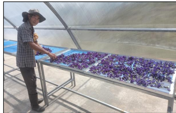
Solar dryer dome to improve dried butterfly peas for farmer group in Lao PDR
